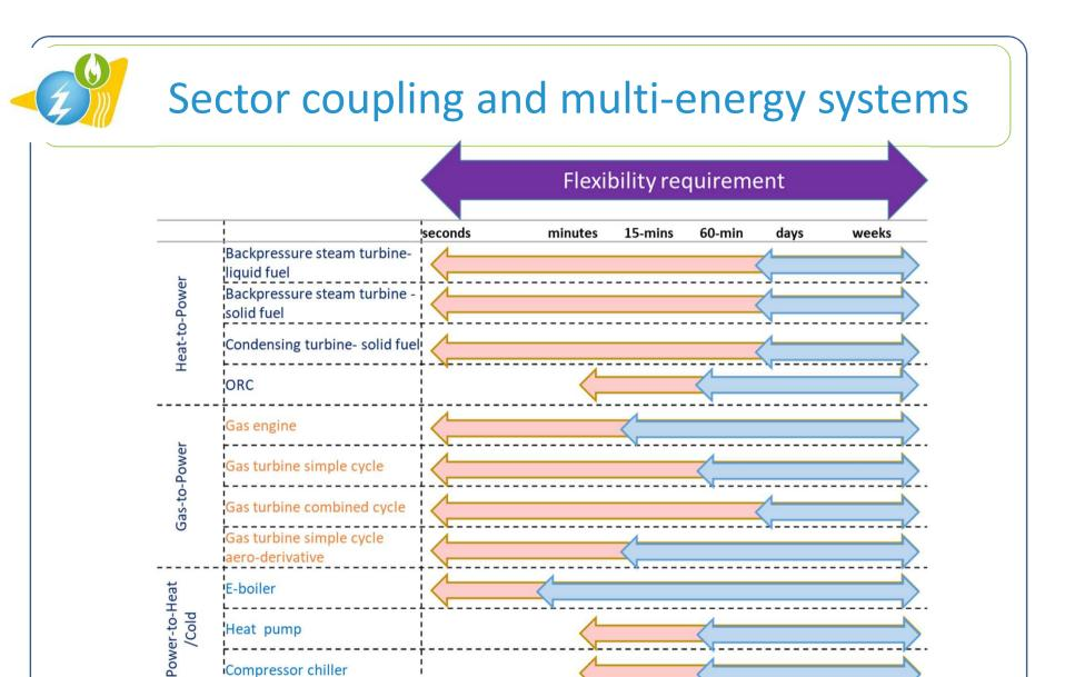
Flexibility options provided by different technologies: orange arrows show capability for running technologies and blue arrows reflect capability including time needed for startup from hot state (MAGNITUDE Deliverable D1.2)
