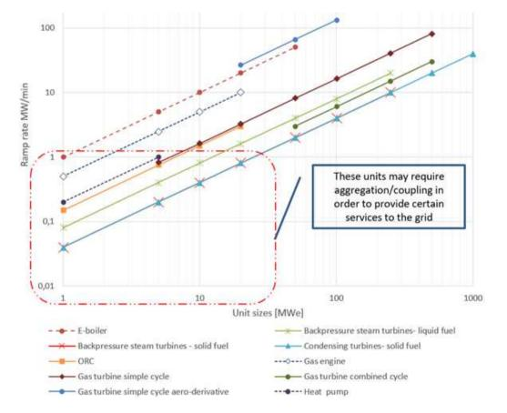
Power range of analyzed technologies and their ramp rates [MW/min]
